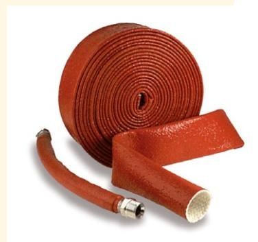
Constructed from a high bulk fiberglass sleeve heavily coated with iron oxide red silicone rubber, Pyrojacket® sheds molten metal splash and withstands intense heat and flame, making it ideal for protecting hoses, cable and tubing in a variety of hostile environments. Withstands continuous exposure to 500°F (260°C), up to 2000°F (1090°C) for 15-20 minutes, and up to 3000°F (1650°C) for 15-30 seconds.
