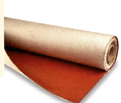
96 oz Pyroblanket is an extreme heavy-duty version of 32 oz Pyroblanket. Utilizing a very thick fiberglass cloth, all the silicone rubber is applied to one side only, creating an ultra-smooth coating on the heavy texturized blanket. Designed to shed molten steel like water off a ducks back, 96 oz Pyroblanket is unique in both form and function.
